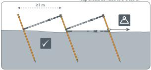
the first ground anchor stake, and the adjustable loop positioned at the base of the second ground anchor stake. Repeat for each subsequent ground anchor stake.
